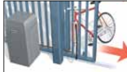
entrapment detection system reverses gate when obstruction is detected
